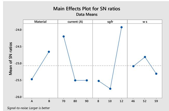
Fig. 4: Main effects plots of SN ratios for Strain
