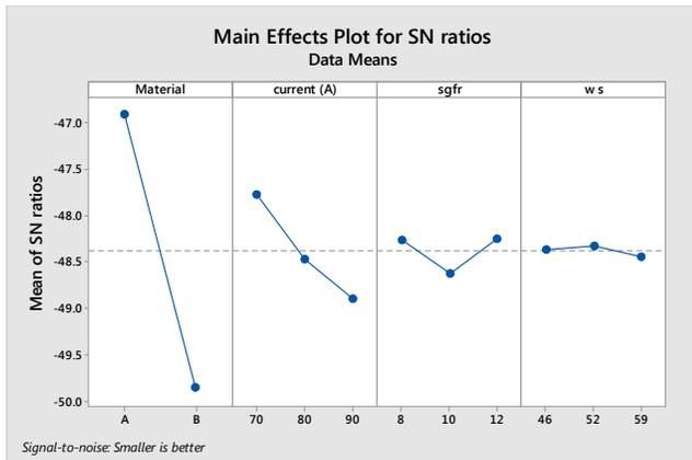
**Fig. 5: Main effect plots of SN ratios for micro-hardness**
