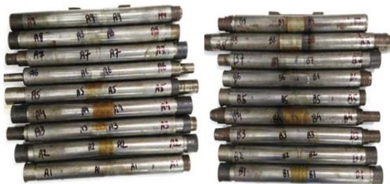
**Fig. 2: Tensile test specimens of pipe weldments.**
